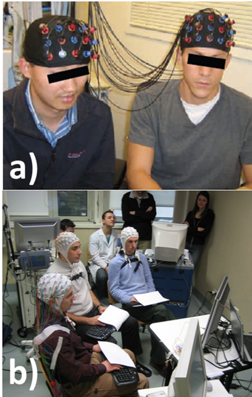
Figure 5. Different hyperscanning devices for hemodynamic and electric modalities The figure shows in the upper part A) the split of the fibers to generate an NIRS hyperscanning device from one single NIRS device; in the lower part B) the EEG hyperscanning setup during an iterated Prisoner's Dilemma task involving three subjects. Figures from Cui et al., 2011 and Astolfi et al., 2011.
